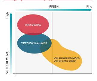
With its tough grain characteristics and ability to generate new cutting edges, VSM ZIRCONIA ALUMINA combines very high stock removal with exceptional toughness in the grinding zone. It is an excellent choice for heavy stock removal applications.
